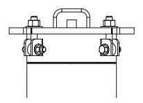
The most economical quick opening closure offered for fabricated strainers with nominal pressure applications. The swing bolt hinged cover uses an O-ring to seal. Easy to open by quickly and easily by loosening the swing bolts until they clear the holding lugs and swinging the head open on its hinge.
