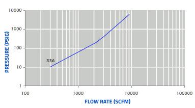
0.65 S.G. and 60 deg F. Based on 2 PSI initial pressure drop.
